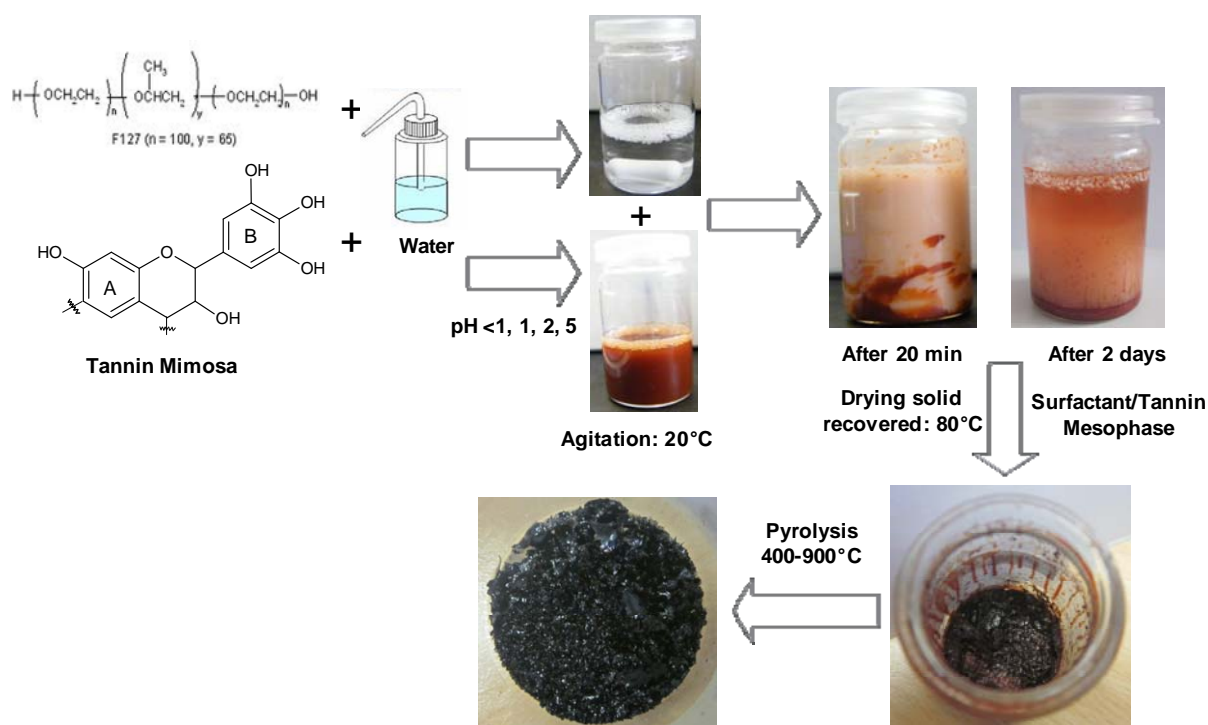
Fig. 91: Schematic approach of OMC's synthesis using tannin and F127.
