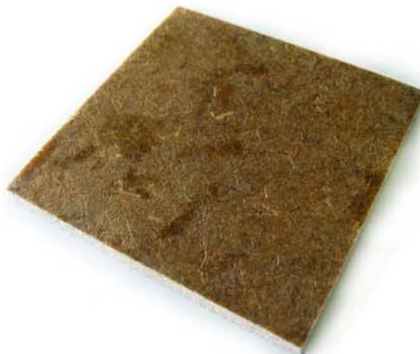
Figure 1. Example of a natural fibres non-woven composite with ESO matrix.
