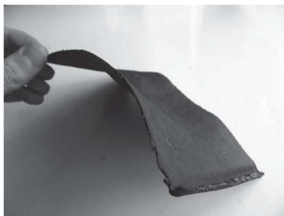
Figure 1 The deformation of a TRF composite.
