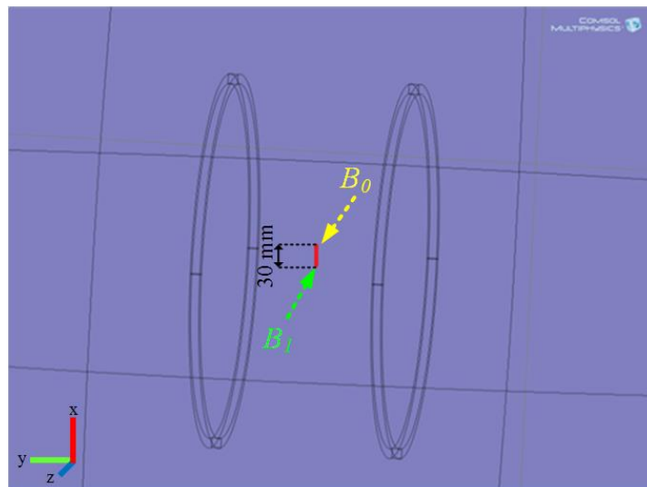
Figure 2.29 Calculation of the magnetic flux density ( B ) along the needle of sensor.
