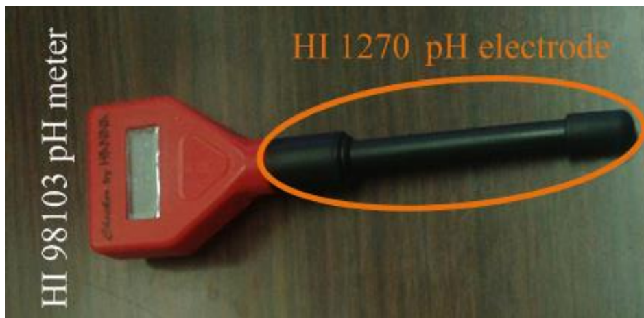
Figure 4.8 The pH meter and its pH electrode.
