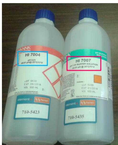
Figure 4.9 The pH 7.01 and 4.01 buffer solutions.
