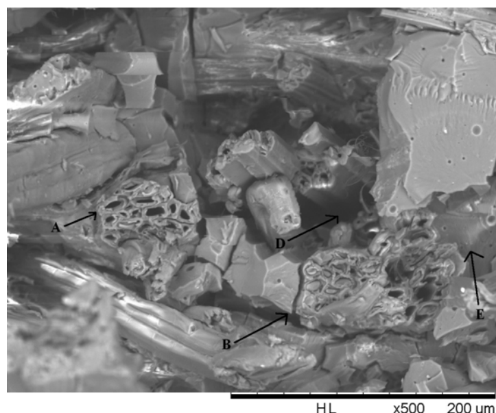
Figure 31 Facies de rupture KENAF T
