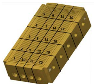
Figure 2-7. Design of the flow field plate from Axane.
