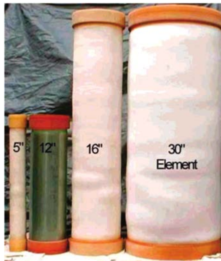
Figure 2.10: Photograph showing the development of hollow fiber modules at Cynara [Baker and Lokhandwala, 2008], from the first 5-in. modules of the 1980s to the 30-in. diameter behemoths currently being introduced. Photo courtesy of Cynara Company (now part of NATCO Group, Inc).
