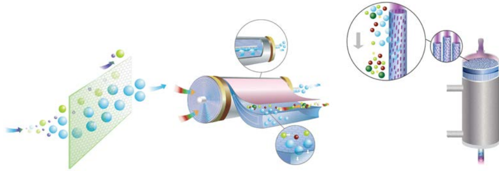
Figure 2.9: Schematic membrane modules. Left: Plate and frame module. Middle: Spiral-wound module. Right: Hollow fiber module ( http://www.co2crc.com.au/ )
