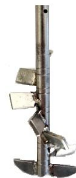
Figure 3. Special helicoidally multi-vane geometry
