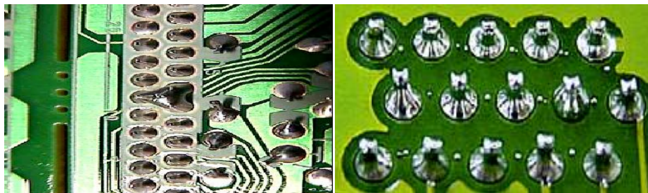
Figure 2.9: (a) too little flux and (b) too much flux
