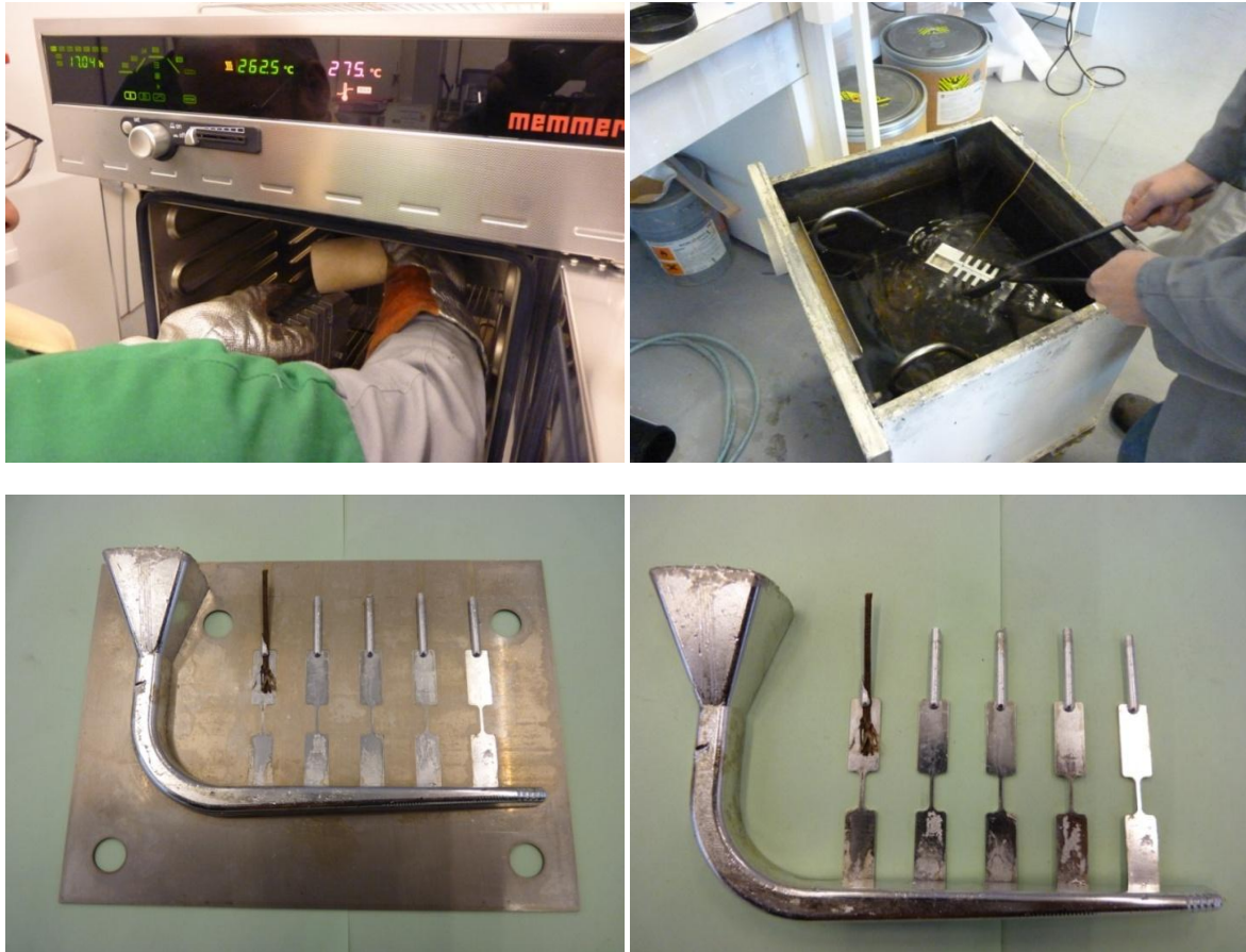
Figure 3.6: Die casting and water quenching of test specimens
