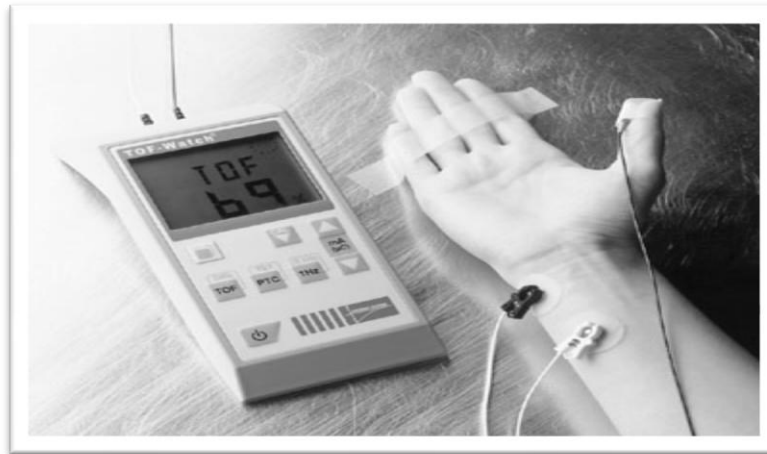
Figure 4: Accéléromyographe (TOF-Watch S®)
