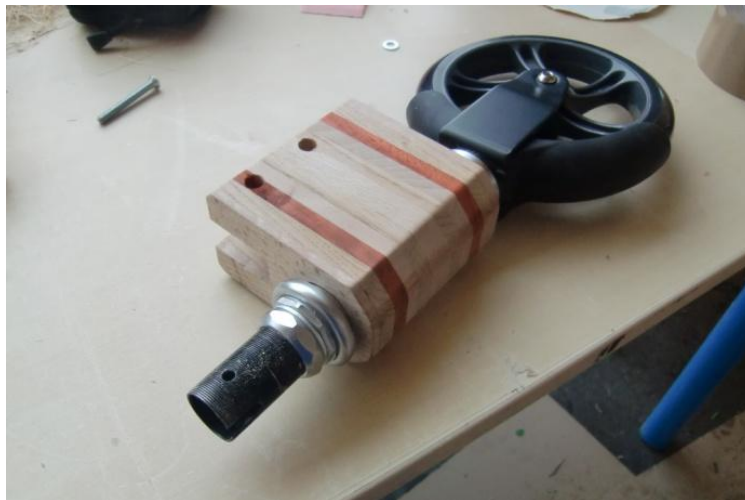
Figure 29: Tube de direction et fourche
